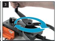
Rolling is achieved by using the winding handle to drive the bar forwards and backwards through the rollers. As this is done with each pass, the long lever is used to gradually increase pressure to roll an ever tighter curve. End stop screw and nut fitted for producing consistent bends and circles/arcs when rolling.
