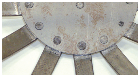
Half Disc connector plate used to make half basket.
